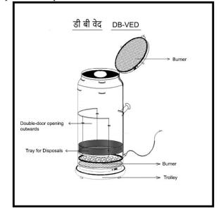
I have designed a special Virus Electrocute Device, the DB-VED, equipped with a couple of hot plates. The sneezing or coughing can be done by lifting the upper burner-lid of the device and placing the head onto the mouth of the device (which provides enough protection from leaking of the virus) and complete the process on the hot plate installed inside. If the process is repeated
