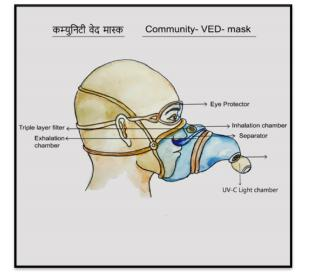
Community-VED-Mask. It has two separate chambers, designated as one for inhaling and another for exhaling. The air inhaled through Inhalation chamber will pass through a triple layered filter, ensuring infection free inhalation. The other chamber of the mask is used to exhale the air. The exhaled air passes through a burner, which will work to electrocute/burn the pathogens and hence, there stands no possibility of contamination of the exhaled air.
