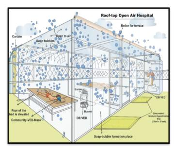
An open-to-air hospital preferably in a countryside or on a rooftop will be a good solution to deal with the problem of Aerosolization and spreading of the virus. The Idea behind is to use UV-rays from the SUN and Soap bubbles for sanitization of Area
