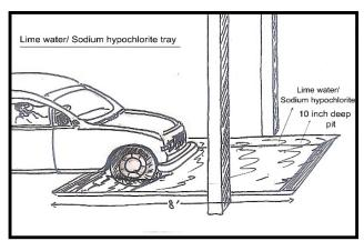
The footwear of a visitor or a vehicle tyre may become a carrier for coronavirus or other pathogens. This can be prevented with lime water or Sodium hypochlorite pits at both entrance and at the Exit of the facility and the patient's room. Similar pits are suggested for cars or other vehicles' tyre treatment on the campus entrance. (figure VI) The Concept and Illustration is by the Author
